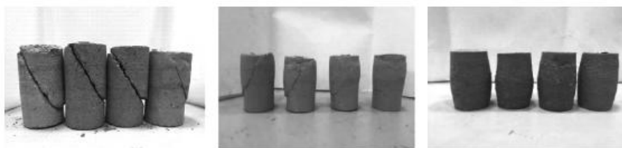
图1 甘孜地区回填土三轴试验试样剪切破坏形态 Fig.1 Shear failure forms of the triaxial test samples of backfilling soil in Ganzi Area
